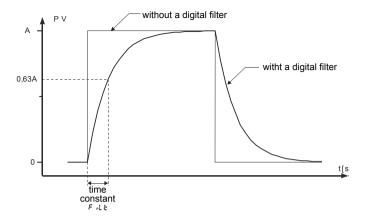
Fig. 25. Time characteristic of the filter
