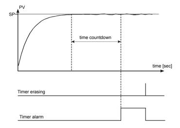
Fig.23. Principle of timer operation
