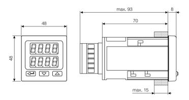
Fig. 2. Controller dimensions.
