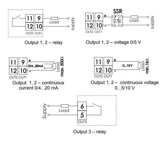
Fig. 7. Control outputs/ alarming
