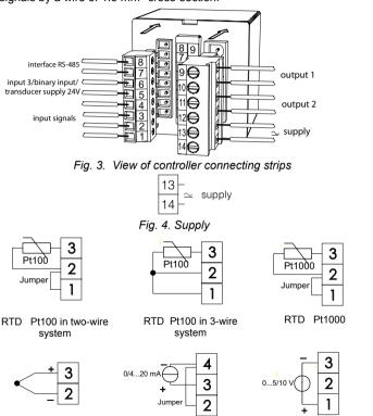
Current input 0/4 ... 20 mA Fig. 5. Input signals
