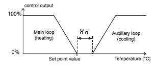
Fig.21. Control with two loops - heating-cooling type
