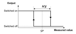
Fig. 16. Operation way of the heating output type
