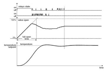
Fig. 18. Three-step step-by-step control with no feedback
